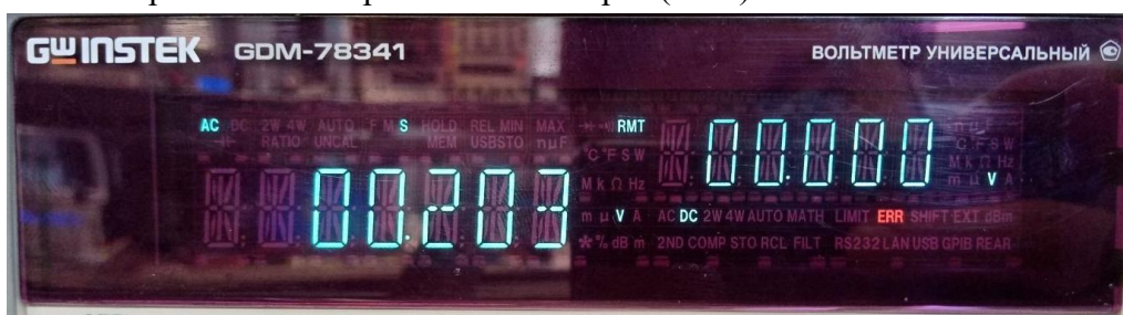
RMT – Remote Control; AC – Alternating Current; S – Seconds; V – Voltage; DC – Direct Current; ERR – Error
